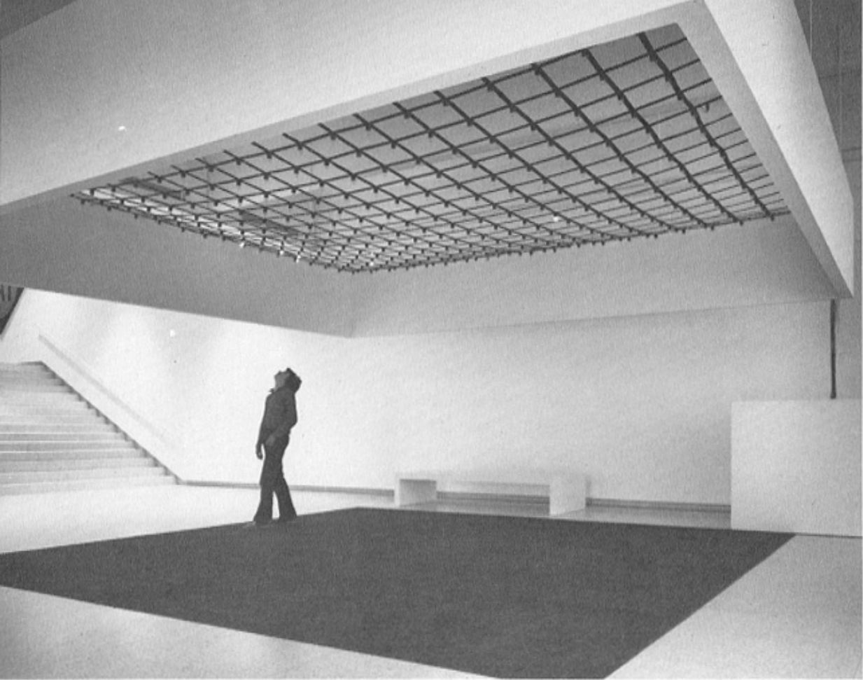
James Seawright. Network III , 1971. Computer-generated environment. The spectator walks over a carpet underlaid with thin pressure plates that activate a pattern of ceiling lights. Courtesy Walker Art Center, Minneapolis. Photo by Eric Sutherland.
